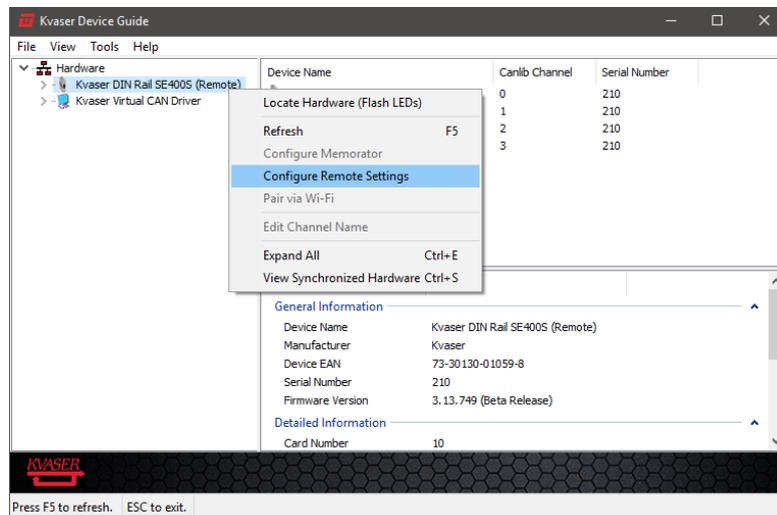
Figure 19: Select device in Kvaser Remote Device Configuration
