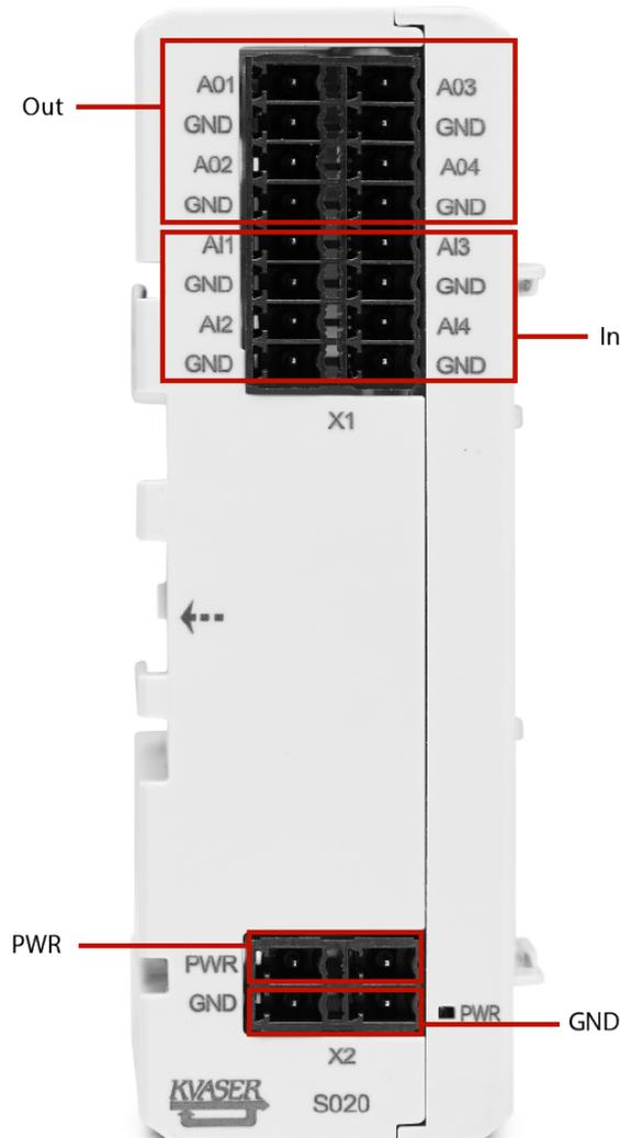
Figure 25: Analog add-on connectors
