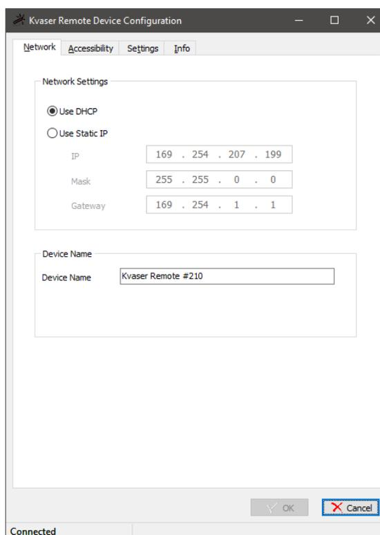
Figure 21: Kvaser Remote Device Configuration network settings
