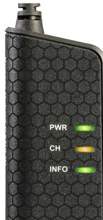
Figure 4: LEDs on the Kvaser Hybrid Pro CAN/LIN.
