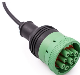
Figure 6: J1939-13 Type II CAN connector
