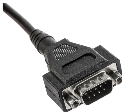
Figure 3: 9-pin D-SUB CAN connector
