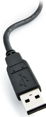
Figure 2: A standard USB type "A" connector.
