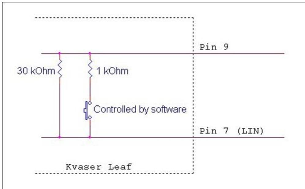
Figure 9: Pull up resistors on the LIN Leaf
