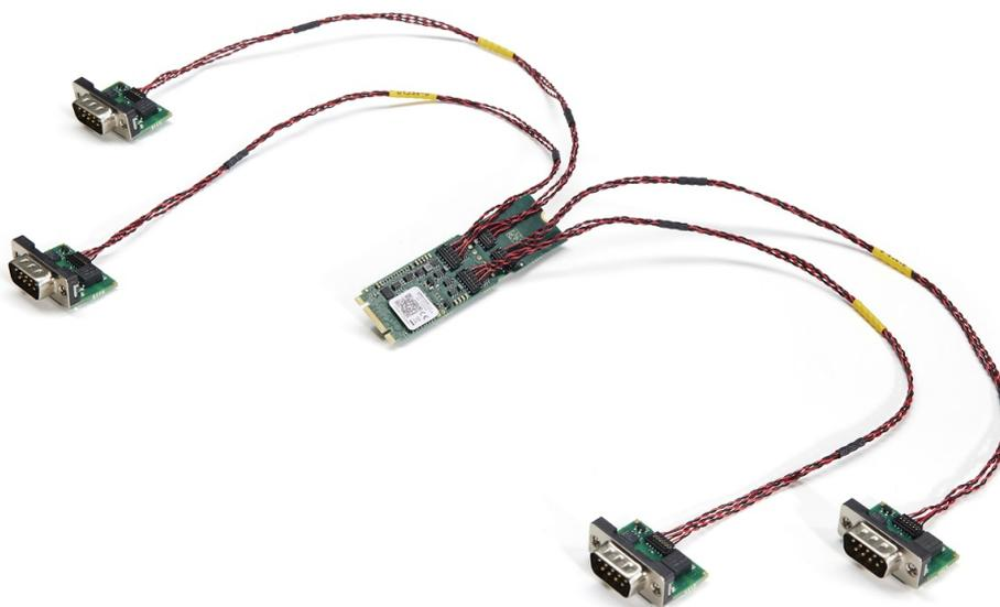
Figure 1: Kvaser M.2 PCIe 4xCAN
