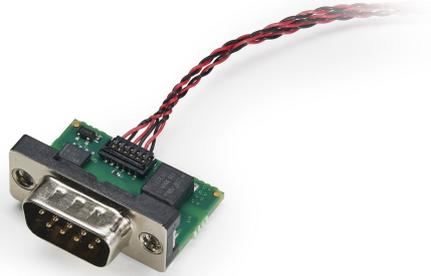
Figure 6: 9-pin D-SUB CAN connector.
