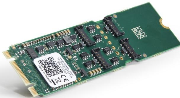
Figure 2: M.2 card of Kvaser M.2 PCIe 4xCAN
