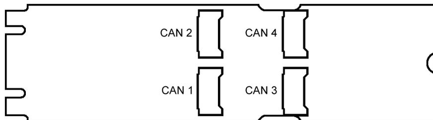
Figure 4: CAN channel layout for the Kvaser M.2 PCIe 4xCAN.
