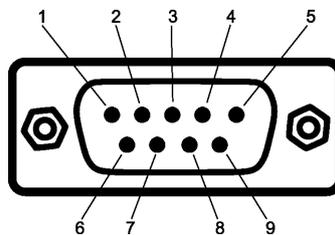
Figure 7: The D-SUB 9 connector pin numbers.
