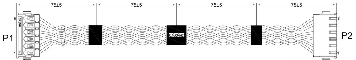
Figure 8: PCB-to-PCB cabling.
