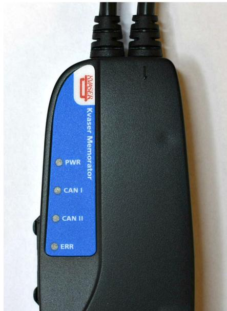
Figure 4: Kvaser Memorator LED indicators
