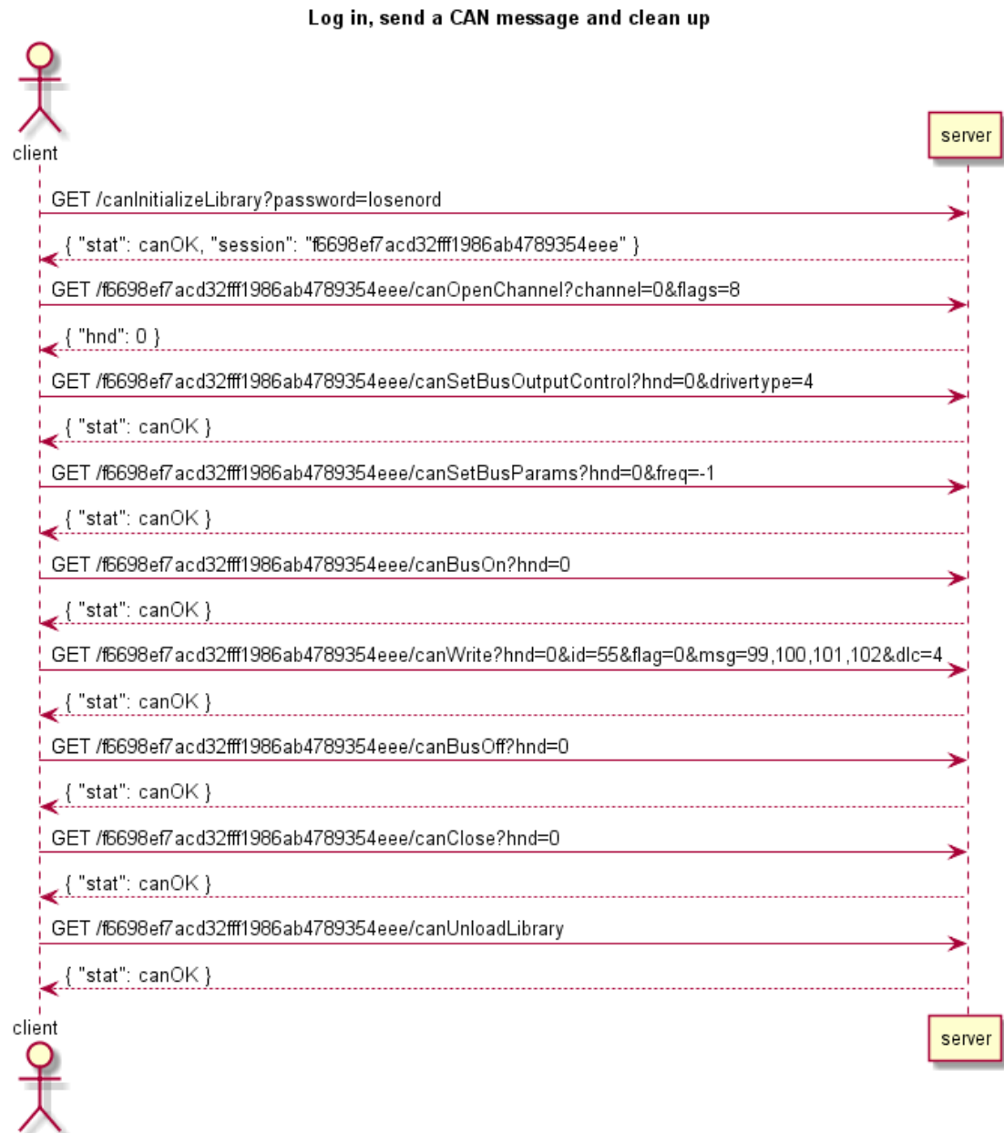
Figure 4: Log in, send a CAN message and clean up
